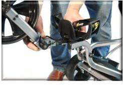
Locate the front wheel assembly and align the assembly with the main frame as shown.
