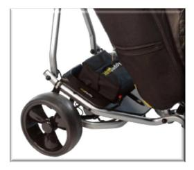
Place the supplied battery into the battery carrier so that the attached lead is close to the connector coming from the buggy. The battery tray is designed so that no strap is needed to support the battery.
