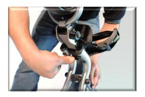
Use the adjacent locking tab to lock the front wheel assembly into place.
