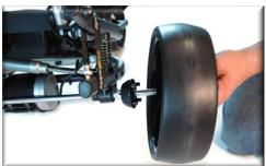
clip in. Slide the wheel onto the axle and onto the four guide pins.
