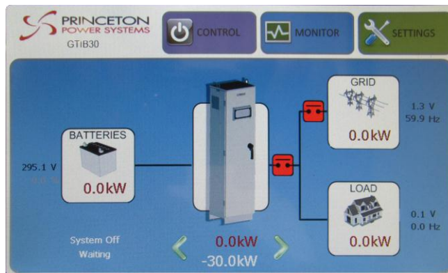
Figure 5: Touch Screen HMI mounted in front door of GTIB-30 enclosure.
