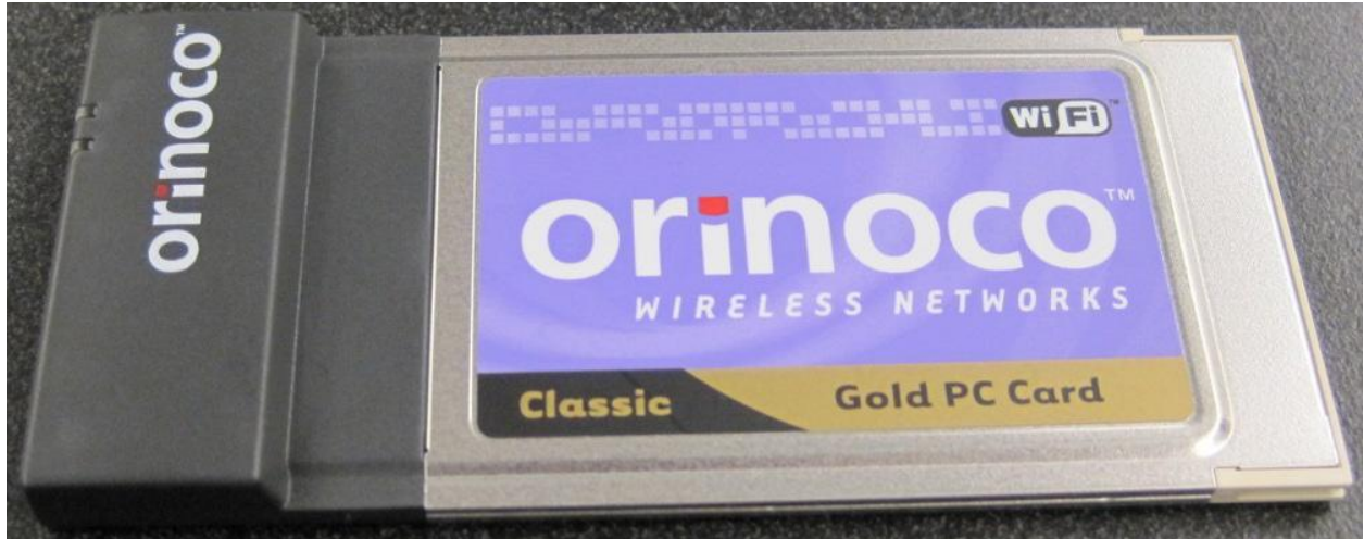
Figure 5 Orinoco Gold Wireless PCMCIA LAN Card
