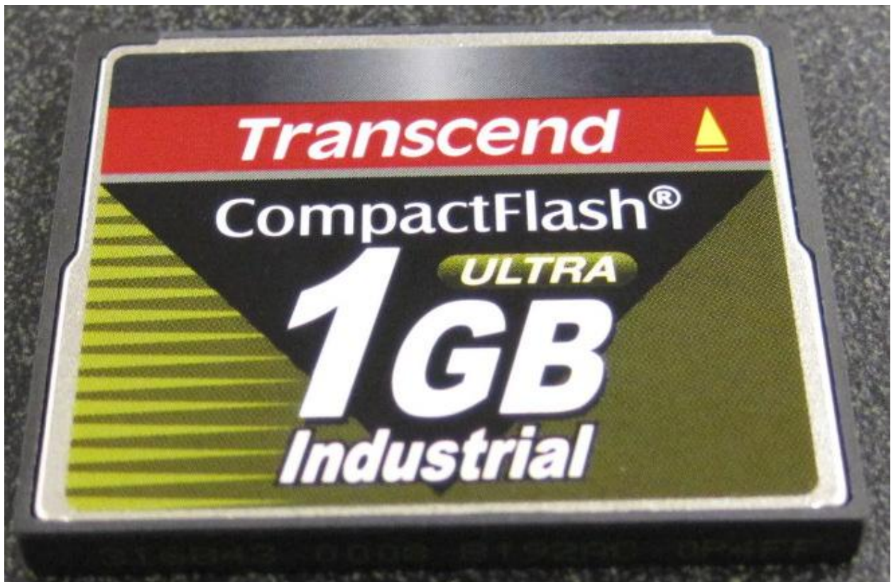
Figure 7 Type I Compact Flash Card.
