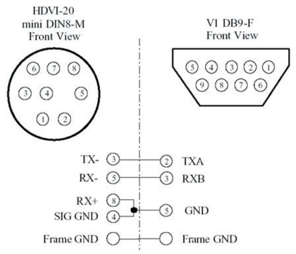
Note: For a true RS422 connection, you can use an adapter made by KK Systems (Part Number K422-99). This adapter connects to the RS232 port on the PC and provides an RS422 connection on the other side. To connect the K422-99 to the HD-SDI to DVI Conversion Box, use a standard RS422 cable (Male DB9 to Male DB9 pin to pin). A true RS422 connection allows for a better connection and longer cables.
