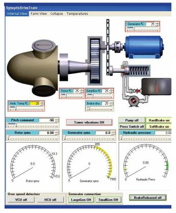
This WTDriveTrain synoptic has been designed to display the most important signals that arrive in the Nacelle emulator, and the signals going out from the Nacelle emulator.
