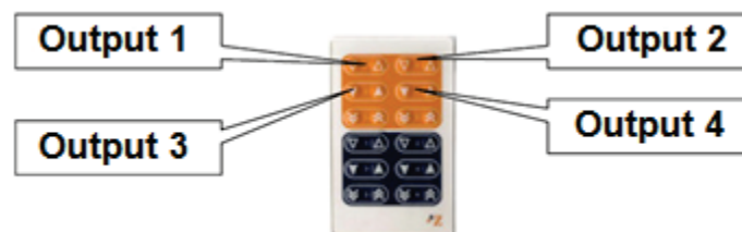
Figure 3 Controlling the outputs from the IR remote
