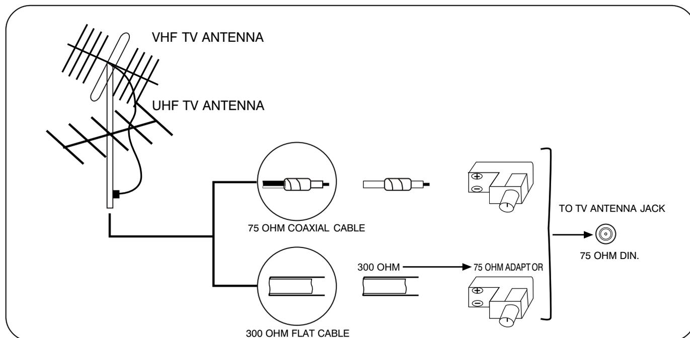
Connect the 75 OHM coaxial cable from the antenna to the antenna jack on the rear panel, as shown above.
