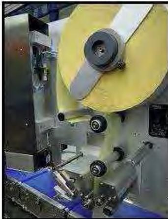
**Fit back the reel holder and begining to guide the paper over the rollers**
