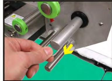
6. Remove the clip which holds the remaining back paper
