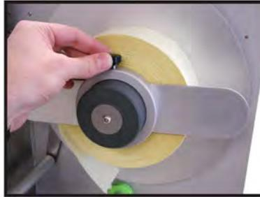
2. Put the new reel in place and screw back
