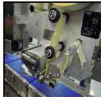
**Hold the paper down with the clip onto the collector roller**
