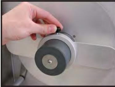
1. Unscrew the securing screw holding the reel of paper.
