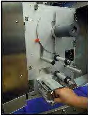
**Turn the metal lever that release the printerhead anticlockwise.**
