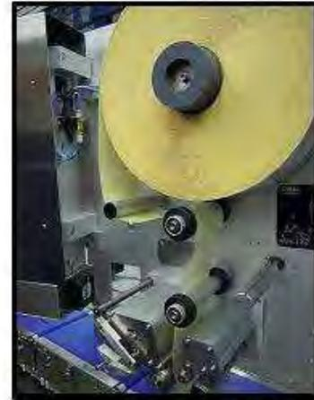
**Remove the safety screw and put the reel in place**
