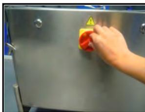
The screen will light up and the start message displays, with memory and printer checks being made. The weigh belts and label belts will operate for two seconds to remove the packages that may have been left on the machine.
