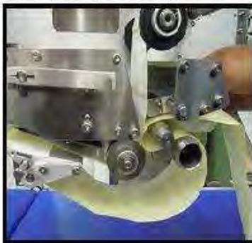
**Guide the paper to the tractor roll follow the direction of the rollers**
