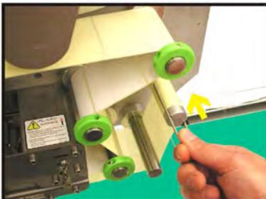
10. Pass the back paper through the low until reach the picker and hold it with the clip
