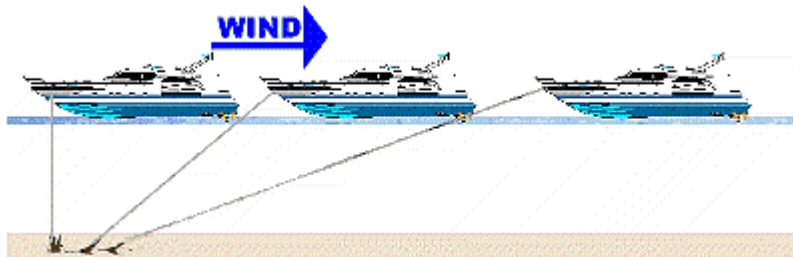
Figure 46: Setting the anchor
