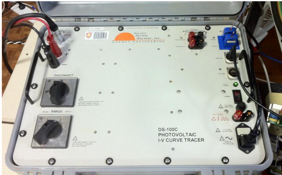
Figure 19 - IV curve tracer used for the test
