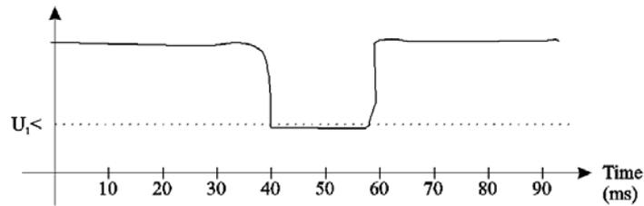
Figure 2.3.4-1. Short voltage sag which is probably not recognized
