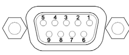
Figure 4.5.1-2. Pin numbering of the front communication port
