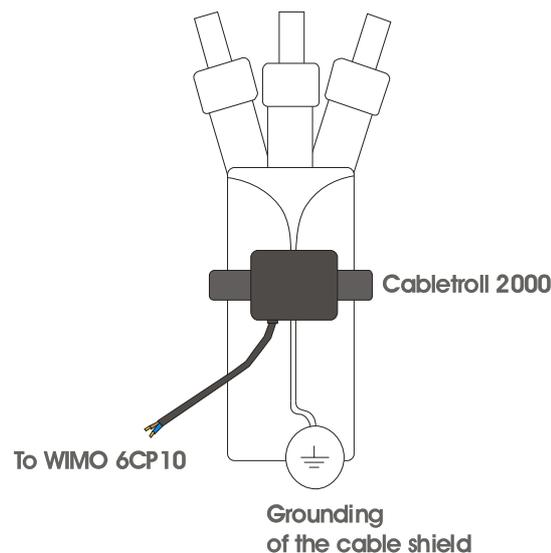
Figure 3.2-1 Cabletroll 2000 attached to the cable of secondary substation
