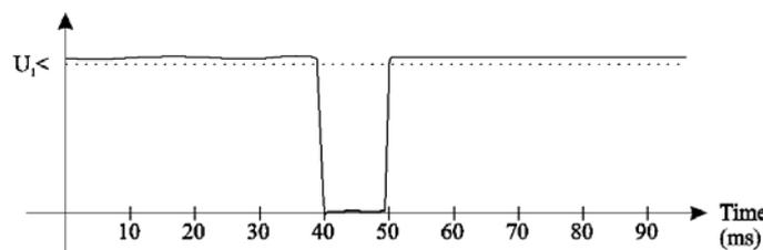
Figure 2.3.4-2. Short voltage sag that is recognized
