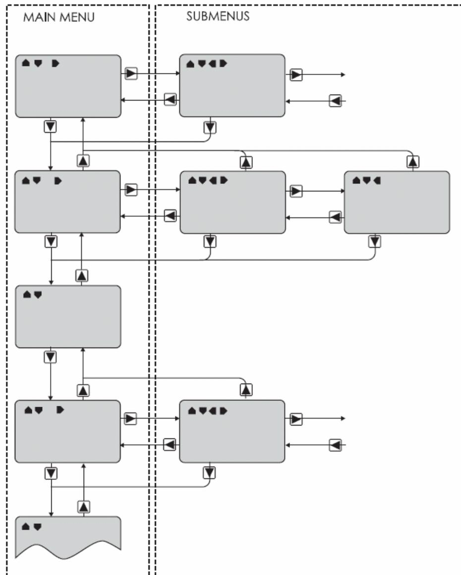
Figure 3.1-1. Principles of the menu structure and navigation in the menus
