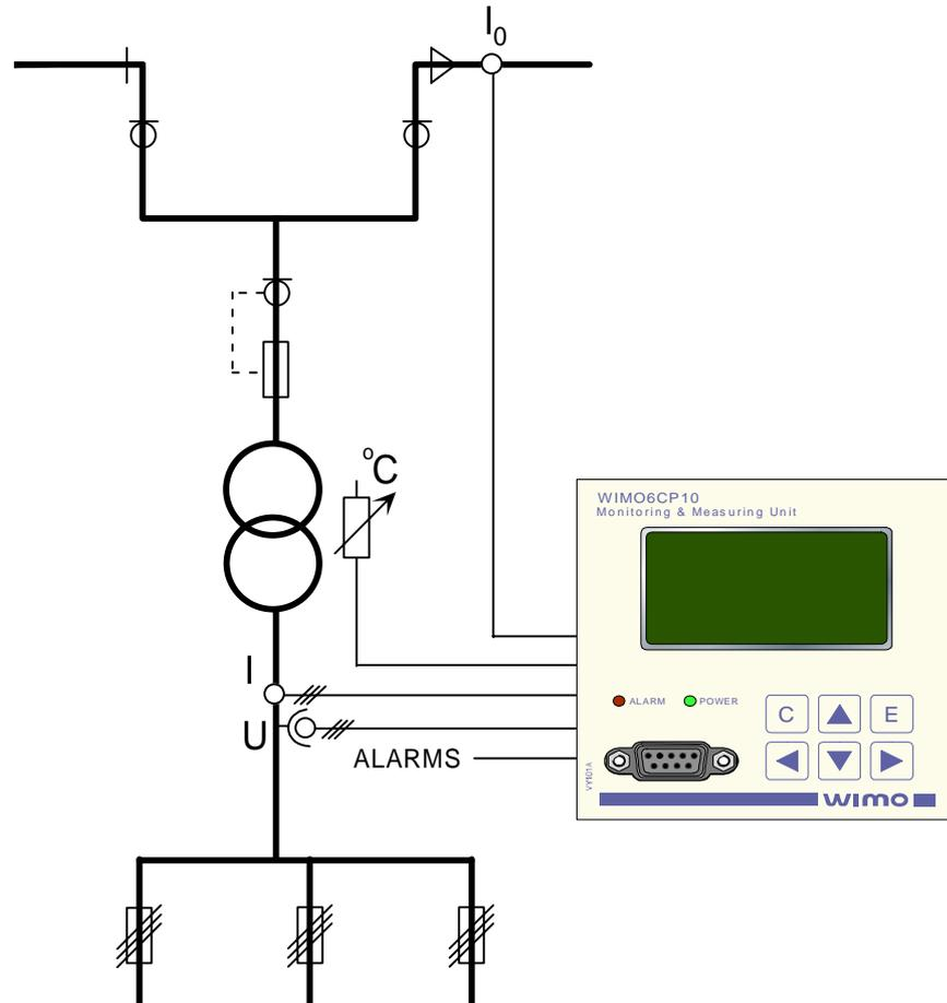
Figure 3.1-1 WIMO 6CP10 used in secondary substation monitoring
