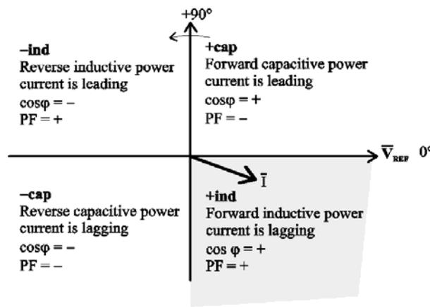
Figure 2.3.2-1 Quadrants of voltage/current phasor plane
