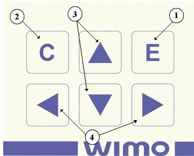
Figure 2.2.2-1 Keys on the keypad
