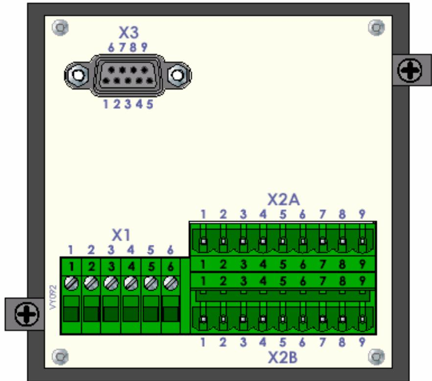
Figure 4.1.1-1 Connections on the rear panel of the WIMO 6CP10
