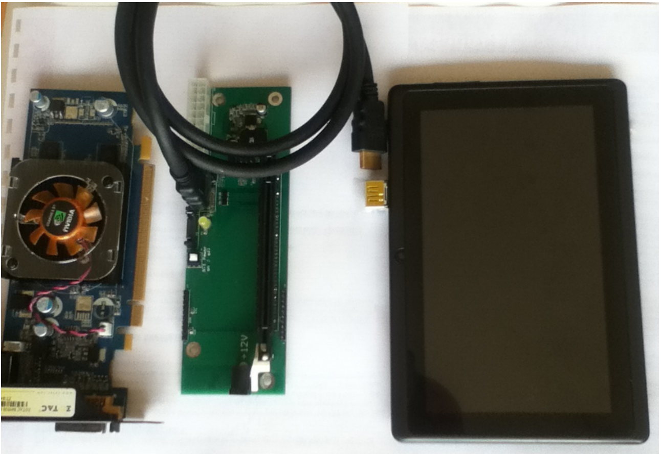
***pic.6 - a tablet + HDMI con., a cable , xprs-px-x16 + PCI Express -x16 card
