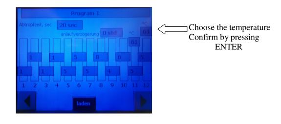
If desired insert, the start time delay for weekends or holidays , this time is set in hours not in minutes. The maximum delay is 4 days .
