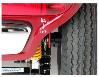
your scooter can still be freewheeled by lifting the front of the unit and pulling, using the base of the tiller as a secure handhold.
