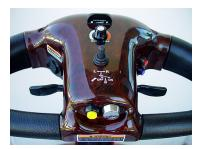
**Hazard Lights** – If your scooter breaks down or you need assistance, press the red button located on the right side of the tiller, just under the forward lever. Once you have received assistance, press the red button again to turn it off.
