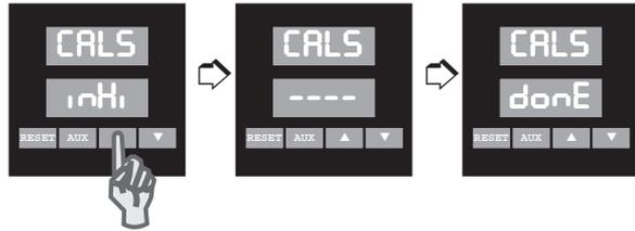
7. Press RESET to exit calibration.
