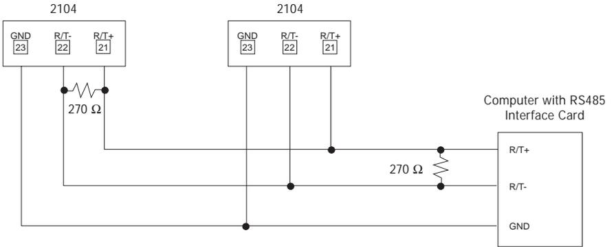
**Note:** 270 Ω resistors recommended across receive line on computer and last controller.
