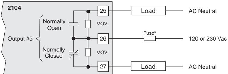
\* Fuse should be sized for the current of Output #5.
