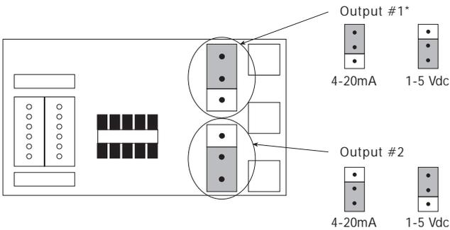
\*All controllers with Analog Output (output codes AR, AT) for output #1 use same 4-20mA/1-5 Vdc jumper positions as shown here.
