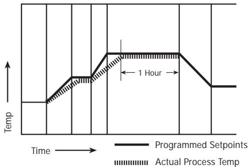
Guaranteed Soak is enabled on the `rSP3 PAGE` by setting the differential band to a value greater than 0. It is adjustable from 1°F to the sensor span.
