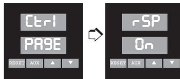
**Note:** The Digital Input or AUX pushbutton can be used to switch between Remote Setpoint and Local Setpoint (see page 57 for setup).
