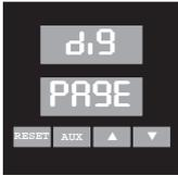
This setup PAGE appears only if the controller is equipped the digital Communications option.
