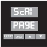
This PAGE appears only when Analog Input is selected, Remote SP is enabled, or Analog Output is enabled on Ctrl PAGE.
