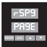
This setup PAGE appears only if Ramp/Soak control is turned on. The Ramp/Soak Enable parameter is the next to the last menu on **Ctrl PAGE, Menu Cont.**
