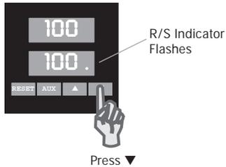
▼ (**Hold**) Stops the program in progress and "holds" the program until the ▲ (**Start**) button is pressed.
