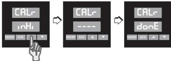
6. Press RESET to exit calibration.
