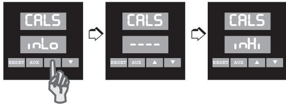
5. When the controller prompts **inHi** in the lower display, adjust the sensor simulator to output the high end of the currently selected sensor span. Sensor maximum ranges are:
