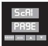
This page appears only if Remote Setpoint and/or Analog Process Output are Enabled.
