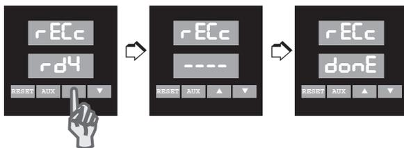
3. The lower display cycles from “----” to “donE”. Press **RESET** to exit the calibration mode.
