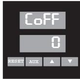
2. Use ▲ and ▼ to set the calibration offset, adjustable from -100 to 100°F.
