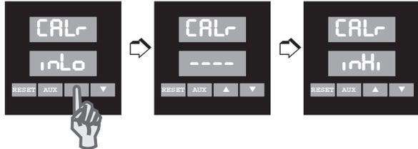
4. When the controller prompts inHi in the lower display, adjust the simulator to output the high end of the currently selected input span (20mA or 5 Vdc).
