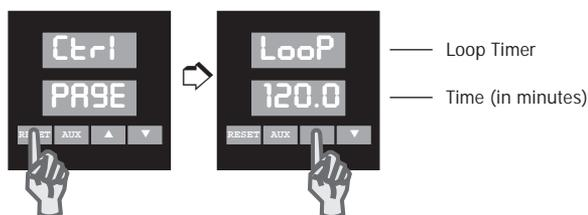
The timer setting should be chosen according to the response time of the system. The minimum time setting should be 0.25% of span divided by the normal load response rate to full ON or full OFF condition (whichever is slower).
