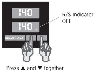
▼ and ▲ together (Stop Pushbutton) return the Ramp/Soak program to the Standby setpoint.
