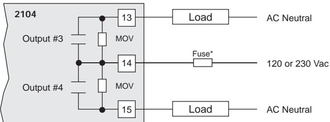
\* Fuse should be sized for the combined current of Output #3 and #4.
