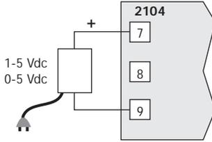
The 2104 has a +24 Vdc power supply which can be used to power a 4-20mA transmitter.
