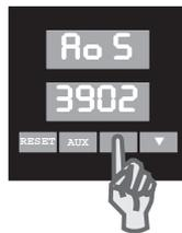
5. Press and hold **RESET** for 3 seconds to exit calibration mode.
