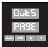
This setup PAGE appears only if the controller is equipped with Output #5.
