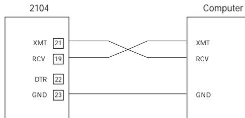
**Note:** The DTR output is always enabled when the 2104 power is on.
