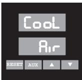
One way to automatically set the PID2 parameters is via the cooling medium parameters. These are setup at menu Cool on the Ctrl PAGE.
