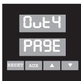
This setup PAGE appears only if the controller is equipped with Outputs #3 and #4.
