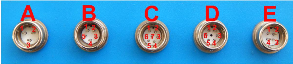
**Figure 4: Connectors pin-out**
