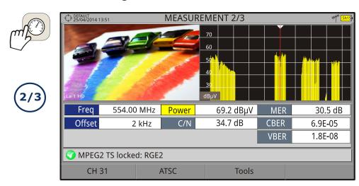
Figure 25. MEASUREMENT + TV + SPECTRUM
