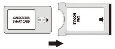
Figure 96. Subscriber Smart-Card and CAM module insertion.
