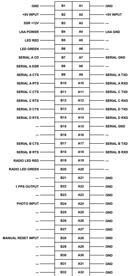
Figure 2.4. Interface Connector Pinout
