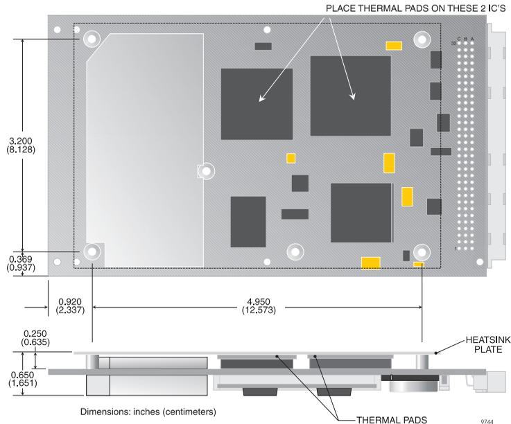
Figure 2.5. ZX-Eurocard Mounted with Heat-Sink
