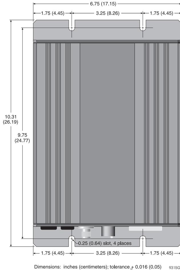
Figure 2.7. ZX-Sensor Mounting Dimensions
