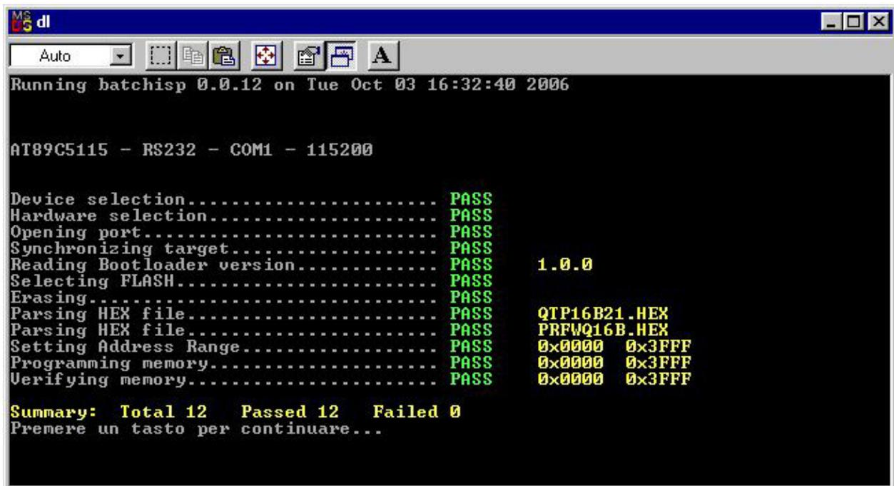
**FIGURE 17: FLASH EPROM PROGRAMMING WITH BASCOM 8051**
