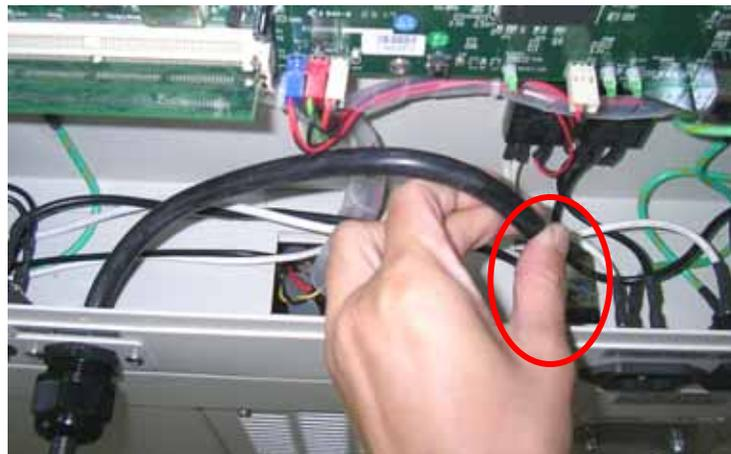
Fig. 2- 72 Insert the Power Cord into the Opening
