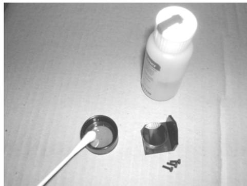
Fig. 7-10 Clean Focus Lens
