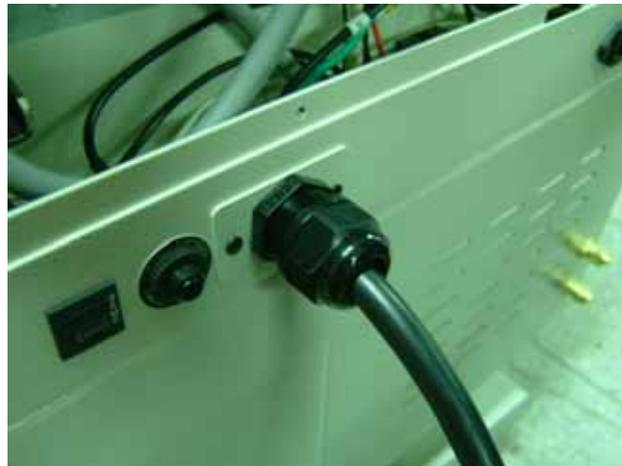
Fig. 2- 61 Lock and Re-install the Wiring Fixing Connector to Laser Machine
