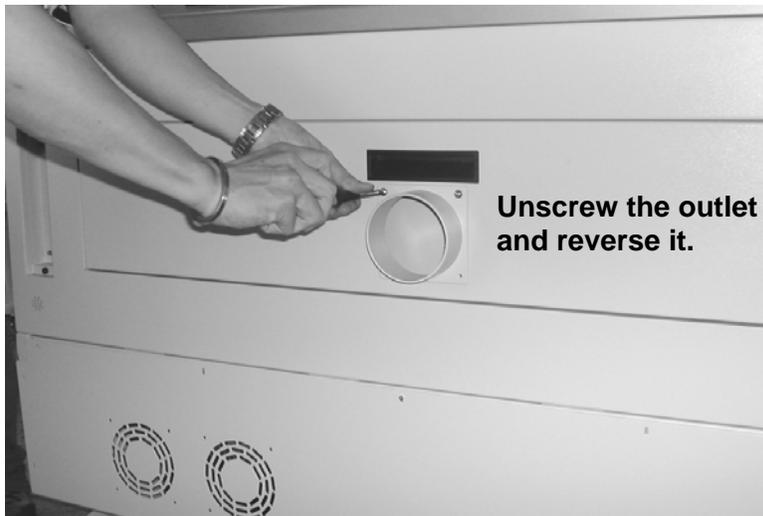
Fig. 3-17 Exhaust System Installation
