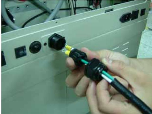
Fig. 2- 50 Insert the power cord through the power fixing connector
