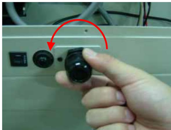
Fig. 2-9 Loosen the Wiring Fixing Connector
