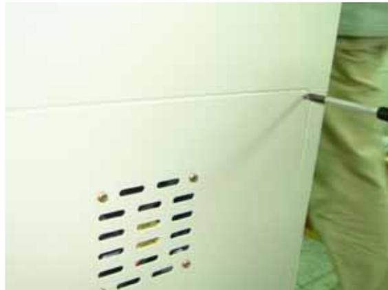
Fig. 2- 8 Unlock the M/B Cover and Laser Cabinet Cover
