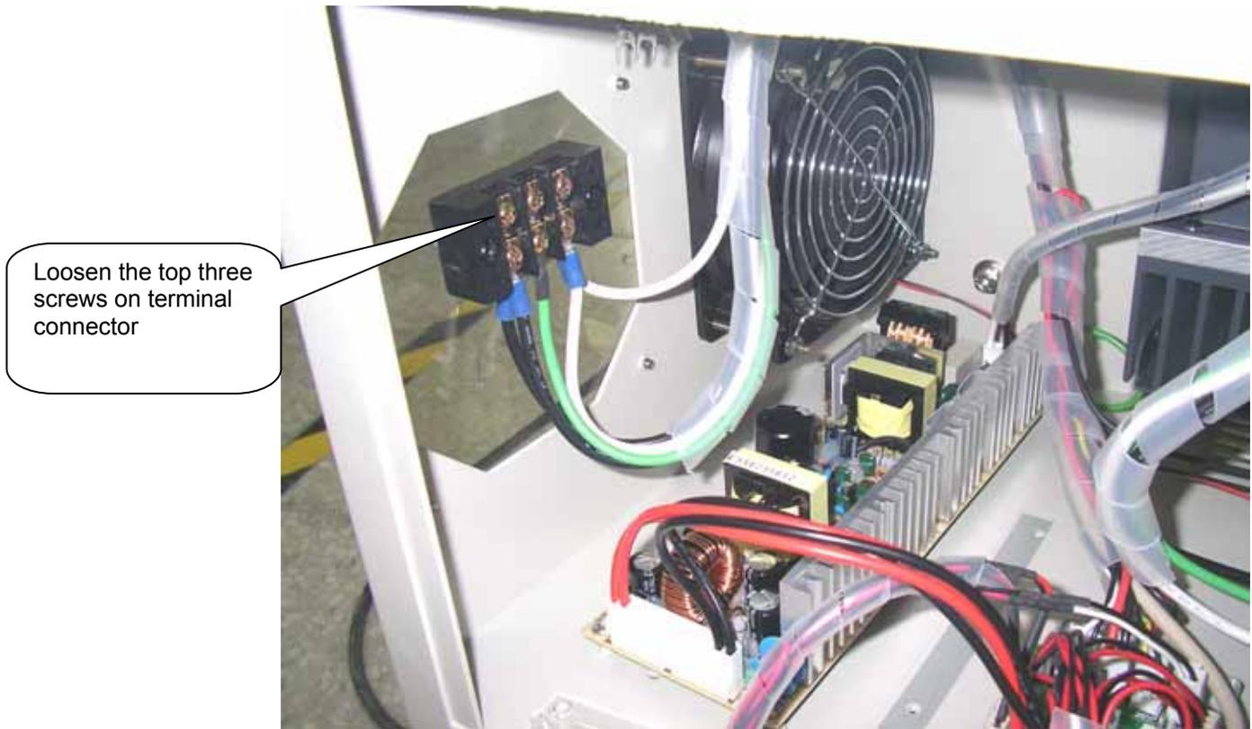
Fig. 2- 83 Loosen the Screw on Terminal Connector
