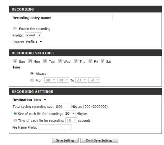
**Total cycling** Please input a HDD volume between 1MB and recording size: 2TB for recording space. The recording data will replace the oldest record when the total recording size exceeds this value. For example, if each recording file is 6MB, and the total cyclical recording size is 600MB, then the camera will record 100 files in the specified location (folder) and then will delete the oldest file and create new file for cyclical recording.
