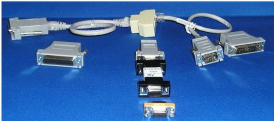
Example of Adapter kit for DB9 (or DB25) cable splitting.
