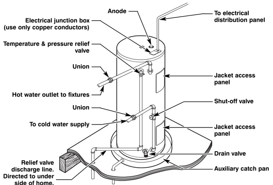
A new combination temperature and pressure relief valve, complying with the Standard for Relief Valves and Automatic Gas Shut-Off Devices for Hot Water Supply Systems, ANSI Z21.22, is supplied and must remain installed in the opening provided and marked for the purpose on the water heater. No valve of any type should be installed between the relief valve and the tank. Local codes shall govern the installation of relief valves.
