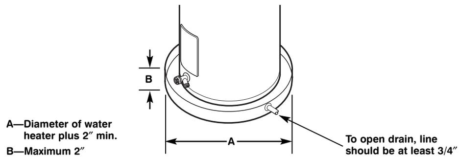
**NOTICE:** Auxiliary catch pan MUST conform to local codes. Catch Pan Kits are available from the store where the water heater was purchased, or any water heater distributor.
