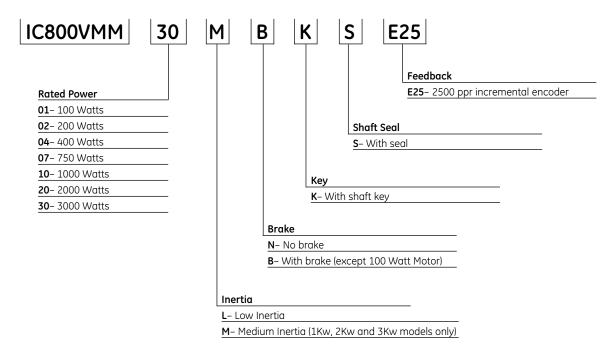
Example: IC800VMM30MBKSE25 is a 3000 watt medium Inertia motor with 2500 ppr encoder, brake, keyway and shaft seal.
