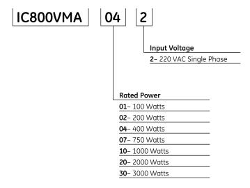
Example: IC800VMA042 is a 400 watt 220 VAC servo amplifier
