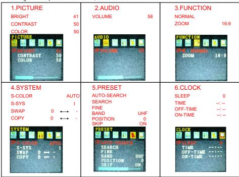
Move to Auto search , press ▶ the system automatically starts to search from 44.00-870.00MHZ and automatically memorize the searched channels. When finish searching, the system will automatically play from the first channel. The screen shows :
