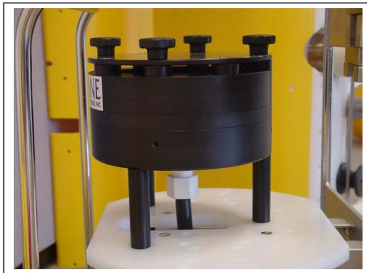
*Figure 2-6: WTS-LV Standard Filter*
