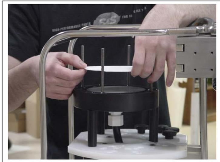
*Figure 5-3: Placing the Filter onto the Filter Holder*
