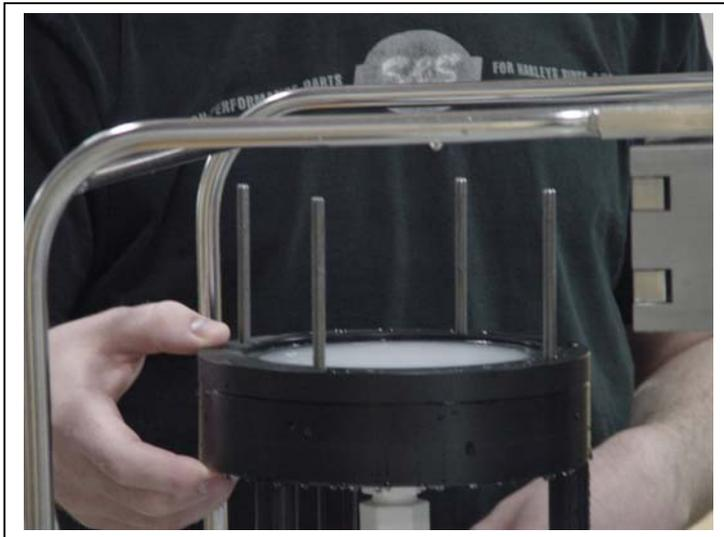
*Figure B-5: Removing Excess Water Below the Filter*
