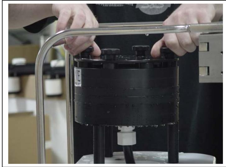
*Figure 5-4: Tightening the Filter Holder Thumb Screws*
