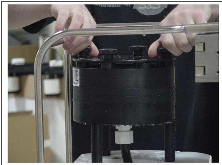
*Figure B-6: Tightening the Thumb Screws*
