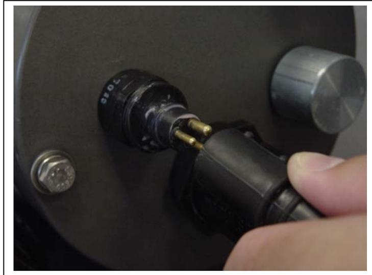
*Figure 2-4: Aligning Cable Connectors with Thumb Bump*
