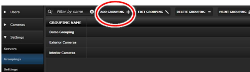
The Groupings (Camera Directory) Element is used to add new camera groupings to the system and to edit or delete existing groupings. To reach the Camera Groupings Element, enter the Administration Module, click the Settings Container, and then click the Groupings Element. The main Groupings screen will display a list of current Groupings. To add a new Grouping, click the Add Grouping control in the Groupings Element screen’s top navigation bar.
