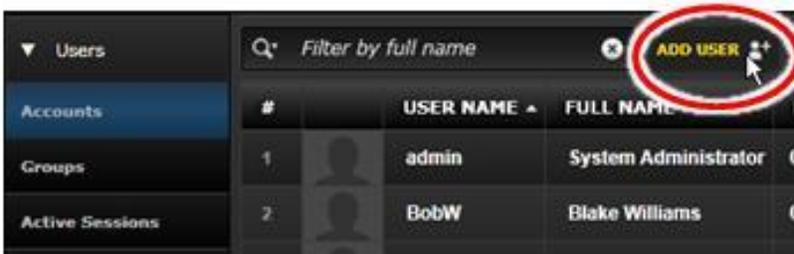
When you click the Add User control, the Add User configuration window will launch. There are a number of configuration screens that will require data. The different screens are listed in the pane at the left of the Add User window. The configuration screens will occupy the pane to the right. As you proceed through the configuration screens, the screen on which you are working will be highlighted in the left pane.
