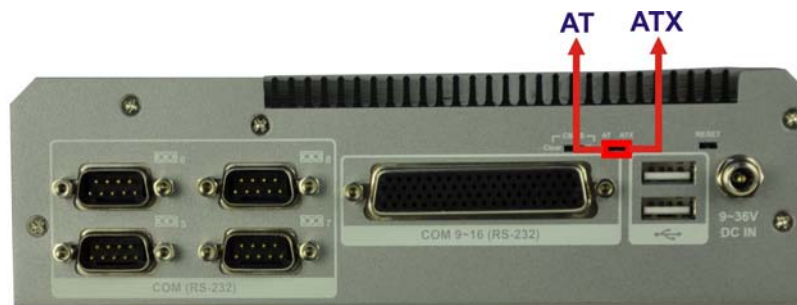
Figure 3-6: AT/ATX Switch Location
