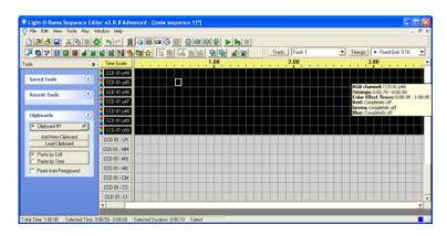
The channels following the RGB channels labeled LR, MM, MS, ... are the control channels for Logical Resolution, Macro Effects and Color Effects.
