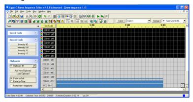
We have set the Color Mode to 17% to select the Dazzle Effect. We have set the Color Speed to 70% to select how fast we want the dazzle colors to change and we have set the overall intensity of the RGB device to 90%.
