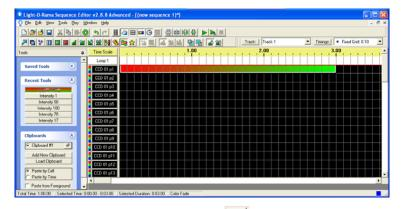
You can click the Play button at this point and the entire ribbon should perform this fade. Because the logical resolution is set to one pixel, all pixels on the ribbon will fade from the color on the left to the color on the right.
