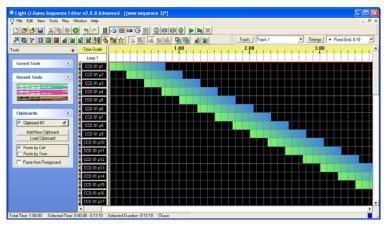
When you click play the device pixels will perform the fade on each pixel chasing away from the controller.
