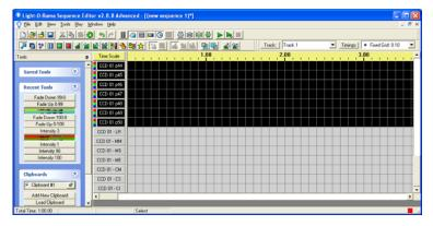
Leave the LR (Logical Resolution) channel off so the device runs at full 50 pixel resolution.
