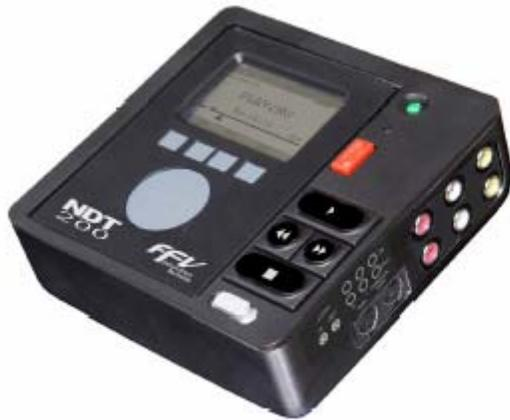
**POWER Switch:** The green pushbutton is the power button, press and release to start the NDT 200™. When the unit is “On”, pressing the power button for 5 seconds will turn the unit “Off”.
