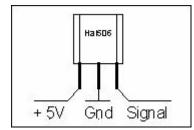
This hall sensor is available from 5 Bears, encased in a 0.25" / 6.35mm aluminum tube, complete with cable and plug for a direct connection to the ECU. It comes also with 2 rare earth magnets for your installation into the compressor spinner nut of your turbine. Please see www.5bears.com for more details
