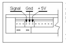
The Inputs port of the ECU is shown here. For a more detailed view, see the ECU Inputs section. The Tachometer input port consists of 3 pins, and the connector is keyed to avoid improper connection. The 3 pins consist of a +5 V source from the ECU, a ground pin, and the signal pin, much like a servo connector.
