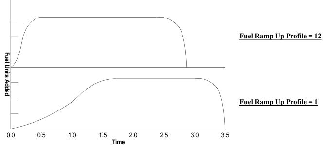
These curves roughly illustrate how fuel is delivered when accelerating from idle RPM to Max RPM. The vertical axis is the amount of fuel added as time passes to accelerate a turbine to max. The overall height of the curve is set with Pump Ramp Up. Pump Ramp Up defines how long the acceleration profile takes from a lower RPM to a higher RPM.
