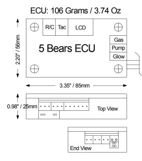
The ECU is encased in a quality ABS plastic box, which is durable and fuel resistant. Connections to the Turbine and inputs are made with Molex "C-Grid" gold-plated connectors which are locking and keyed. The pins are a standard 0.100 inch spacing and will accept many R/C styled connectors. If this is done, you must respect the polarity of the connection.
