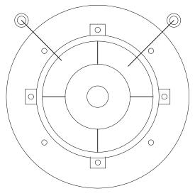
the average temperature, and thus work done, by the turbine wheel. Likewise, longitudinal changes in tip position will produce dramatic variations in measured EGT. I have spent many weeks of testing, and despite this rather non-precise approach, this is the best way to set an EGT probe for correct use in these turbines.
