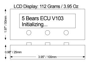
The LCD Display is both light and compact. It does not need to be connected for any portion of the flight, including startup. It is needed, however, to program the ECU and to display post-flight data, and if desired, it may be connected permanently to display all of the normal turbine parameters.
