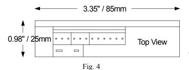
The inputs for the ECU are located on the top edge of the case. Three C-grid connectors accept R/C, tachometer, and LCD Display inputs. The fourth connector is a standard miniature type-k thermocouple jack for the EGT probe.
