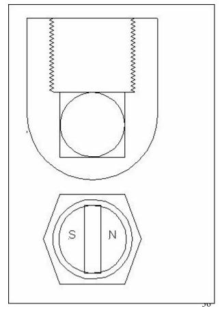
An alternative to the dual-magnet nut shown previously is this compressor nut created for a single, disk magnet. The magnet's diameter is measured, and the nut bored as deeply as possible with a diameter identical to the measurement. The magnet is then pressed into the bore; since the magnet disk has a thickness, the edges of the magnet will "swage" or form a channel for each edge and nicely self-center.
