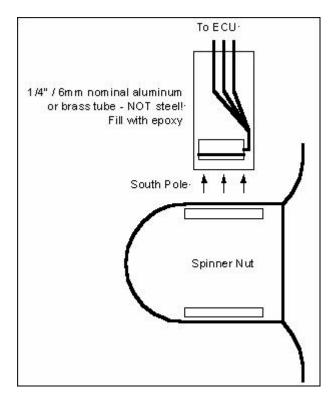
A typical positioning of the tachometer is shown here. After soldering the three wires to the chip (26 gauge servo wire works fine), the leads are bent and the wire routed up through a brass or aluminum tube. Don't use steel or any other ferrous metal, which would interfere with the magnetic signal! Fill the tube with epoxy, "potting" the sensor in place.
