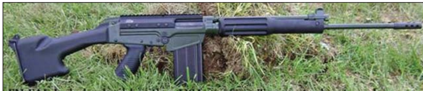
FN-FAL Imbel rebuild with a DSA receiver, Tapco stock set, and Duracoat (FN-Green)
