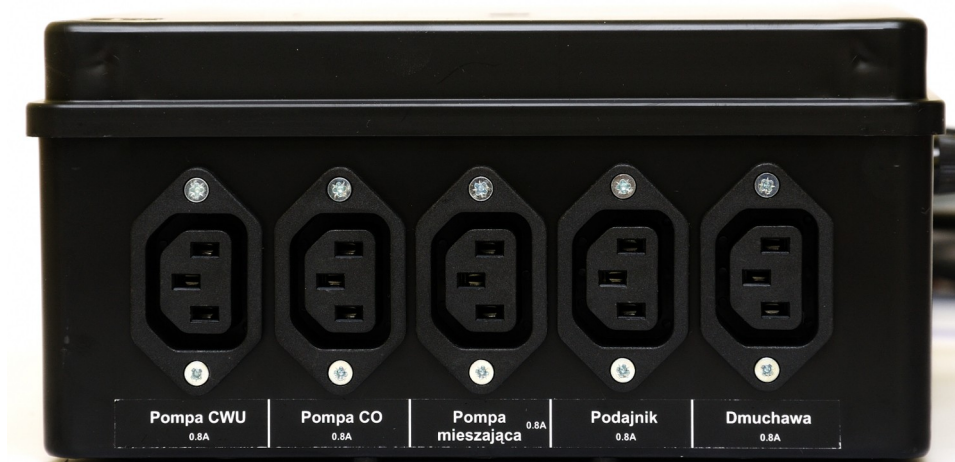
Fig. 5: Housing wall with power outputs
