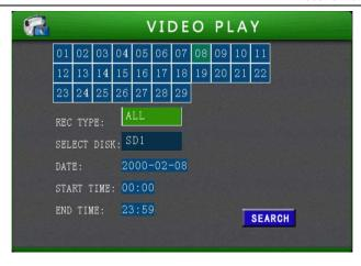
Calendar: green means normal video recorded, red means alarming video recorded and blank means no video recorded.
