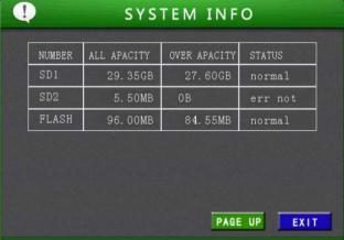
Press INFO and you can quick launch the menu to view the situation of module, connection to center server, alarm, version and storage disk.
