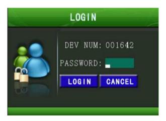
The device support 2 USER level for login: user, admin. The "user" can only check but with no right for parameter setting which "admin" has.
