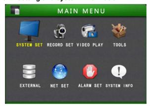
System setting: system management setting, including sub menu as following: time, user, switch and terminal setting.
