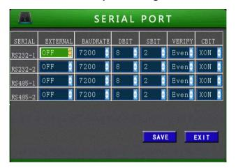
Select external equipment at serial ports and parameters as baud rate will be default. If the external parameters disaccord from default ones, you can modify them manually and save them before you exit.
