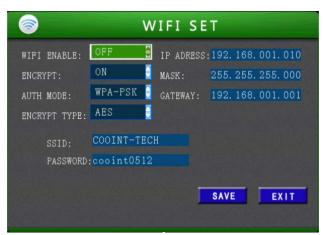
The parameters of WIFI module connect to wireless router, static IP supportive, and you will set IP and AP in the same network segment manually.
