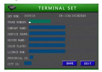
• Device number: there is an unchangeable serial number of the MDVR, which is the only ID when reporting to the surveillance center
