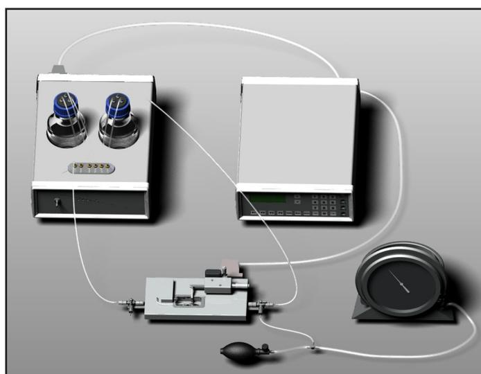
**Figure 4.7** Illustration of set up for pressure transducer calibration
