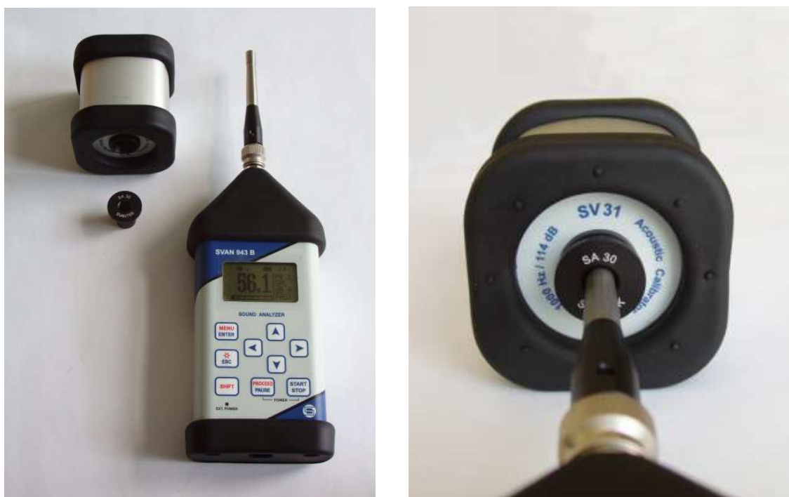
Picture 3. Calibration of the SVAN 943B sound level meter with a ¼” measurement microphone
