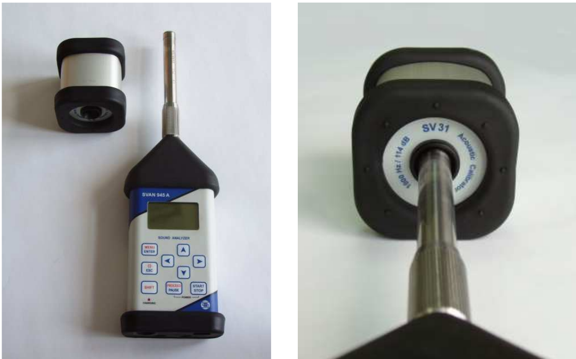
Picture 2. Calibration of the SVAN 945A sound level meter with a \frac{1}{2} " measurement microphone
