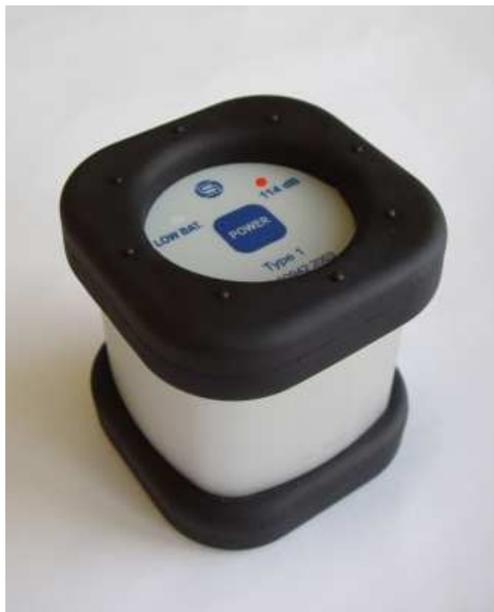
Picture 4. The top view of the SV 31 calibrator with one burning diode
