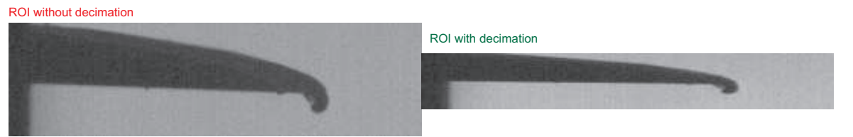
Figure 5.10: Example of decimation 2 on image of injection needle
