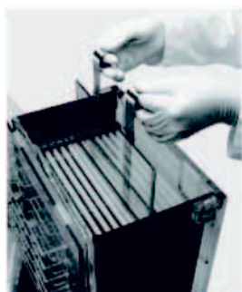
Figure 4-3. Using the cassette removal tools.
