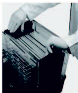
Figure 4-4. Removing cassettes by hand.
