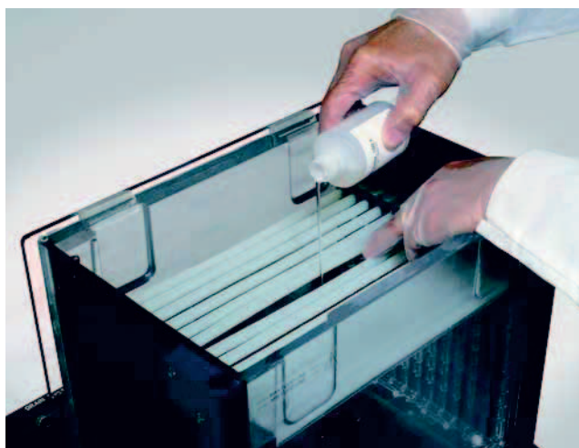
Figure 4-1. Spreading the tubing elements apart with one hand while pouring the solution with the other (to avoid pouring the DIGE buffer onto the tubing).
