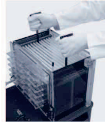
Figure 5-1. Using the buffer seal removal tools
