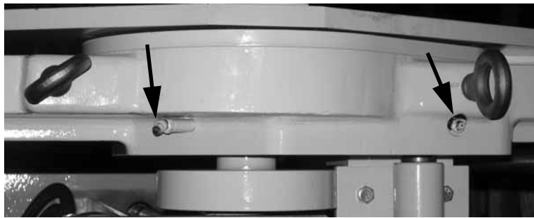
Figure 6-4. Grease the two fittings on the cutting gear housing.
