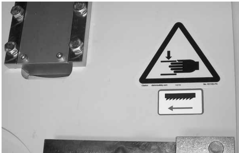
Figure 2-4. The crush hazard warning label and blade direction label are attached on both sides of the saw bow.
