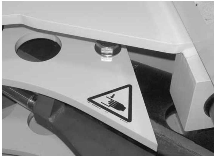
Figure 2-3. The crush hazard warning label is attached in 2 places on the saw frame assembly.
