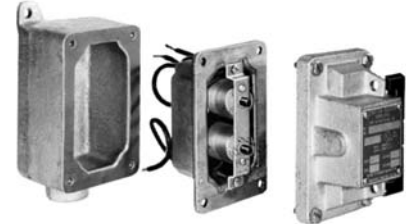
EDS factory sealed rocker arm push button control station—shows separate sealing chamber and device construction. Rocker arm has holes for lock.
