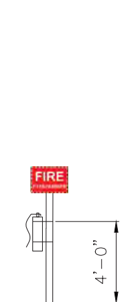
FIRE EXTINGUISHERS TYPICAL
