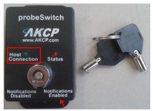
When connected to the unit and the key is in the "Notifications Enabled" position here.
