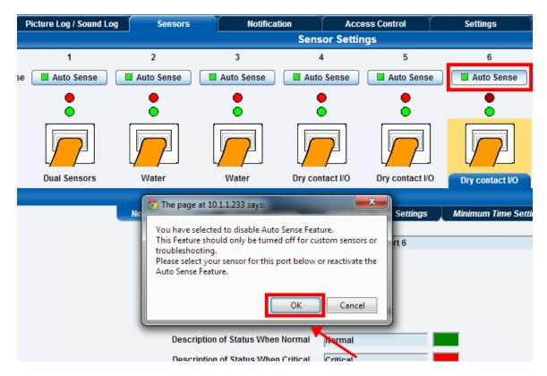
Next we need to turn off the auto sense for that port we have the probeSwitch connected to as shown in the screen shot above.
