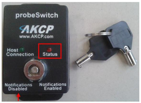
When connected to the unit and the key is in the "Notifications Disabled" position here.
