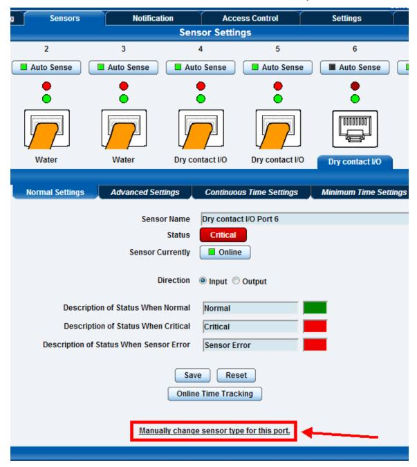
Now we will manually configure the probeSwitch by first clicking on the "Manually change sensor type for this port" link as shown in the screen shot above.
