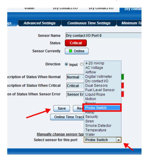
Then choosing the "Probe Switch" from the list of sensors as shown in the screen shot above and clicking on the "Save" button.
