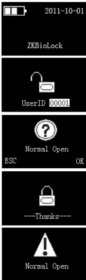
1. Press the **Start** key to display the initial interface. As shown in figure 1 on the left. The **Fingerprint Collector** is in active state.
