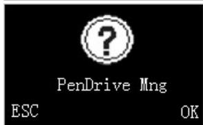
2. Move the **Band Switch** back of the fingerprint lock to the middle position, and then press **OK** key to enter the query interface of **PenDrive Mng**, as shown in figure 2 on the left.
