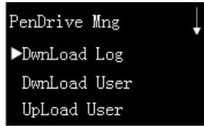
**Note:** When the battery voltage is too low, the user cannot enter the **PenDrive Mng** interface, and the green indicator light for **Fingerprint collector** continuously flickers. Please press **ESC** key for 5s to turn off the battery.
