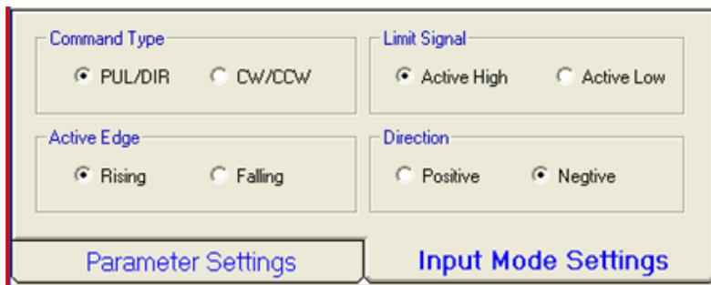
The user can set the command's active edge, direction logic, active level of the Enable and Alarm signal, position following error, electrical gear and motor pole pairs according the motor and application.
