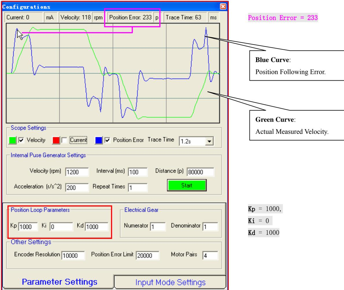
**Step 3:** Increase  $K_p$  and  $K_d$  to maximize the system stiffness or minimize the position error until the motor noise/vibration can not be accepted. To activate the noise/vibration, sometimes you need to give a disturbance to the load by either clicking the **Start** button or trying to push/pull the load. In this example, we give  $V_p$  400, 800, 1000 and find that the noise/vibration at  $V_p=1000$  can be accepted. So we stop increasing  $V_p$ .
