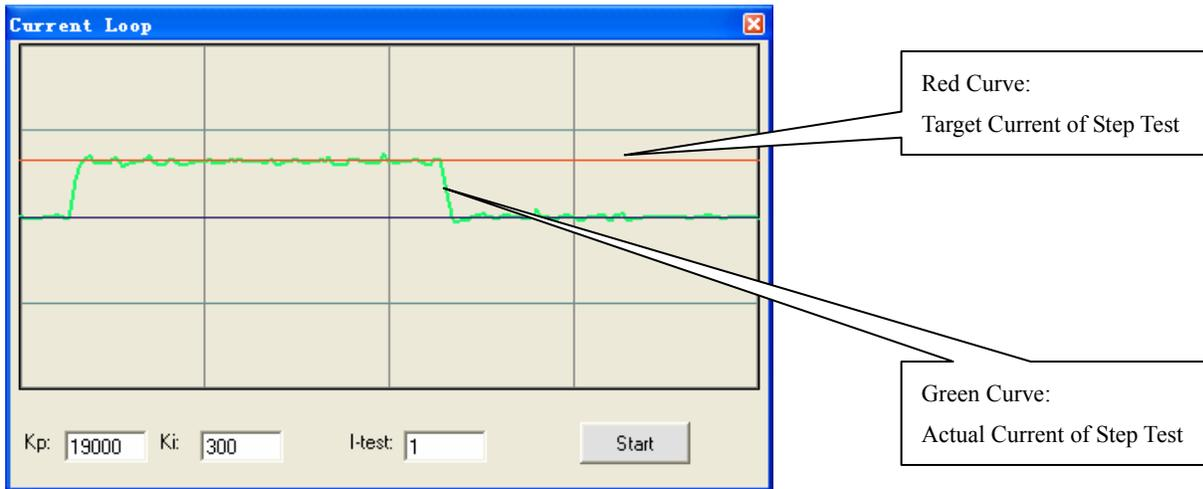
Click **Drive->Current Loop** to open the current loop tuning window. It is used to configure current loop parameters according to different motor. In the tuning window, the user can adjust the proportional gain, integral gain and test Current.
