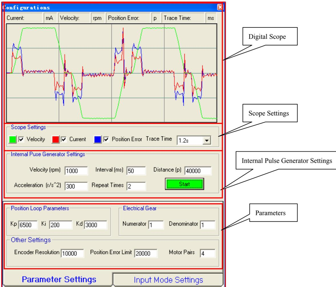
Click **Drive->Configurations** to open the configurations window. The user can adjust the position loop PID parameters and check the result by clicking the Start button. A build-in Pulse Generator performs trapezoid velocity motion and the Digital Scope displays the motor's actual velocity, current and position following error. You can also set the electrical Gear, encoder resolution, position error limit and motor pairs in this window.
