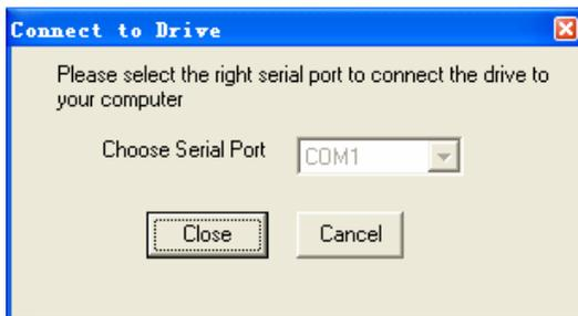
Connect to Drive window appears at start-up. You can open it by clicking **Drive->Connect To Drive** any time. Select the right serial port and click on the Open button. The software will try to connect to the drive and read the settings. It may take several minutes. Please wait.
