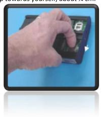
While the clip is slid towards you, pull it upward and outward. The end, closest to you, is on a hinge. Insert the SIM, so that contacts are facing down, close the clip, and close the cover panel.
