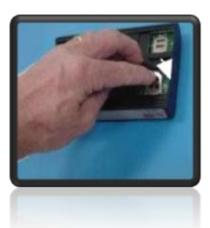
The SIM card slots in each port are numbered from the antenna down as #1, to #4.
