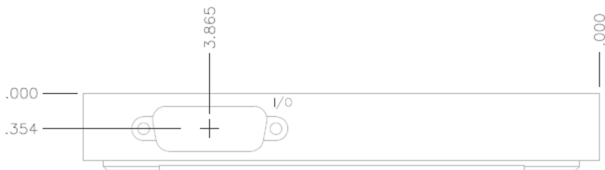
Figure 9: IDAN Back Panel Drawing
