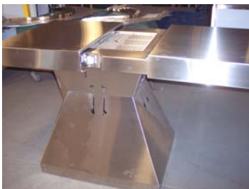
Incorrect-only one shelf open!
