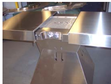
Incorrect- shelves not fully open!
