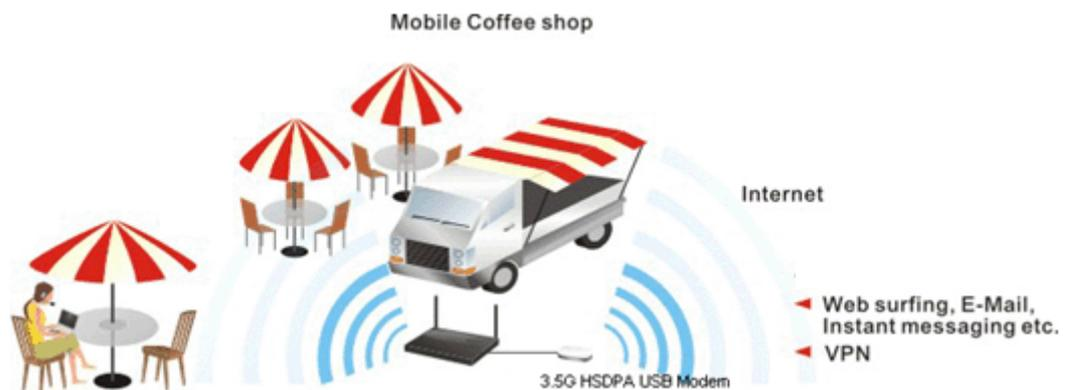
After connecting into the router, 3G USB Modem will be regarded as the second WAN port. However, the original Ethernet WAN1 still can be used and Load-Balance can be done in the router. Besides, 3G USB Modem also can be used as backup device. Therefore, when WAN1 is not available, the router will use 3.5G for supporting automatically. The supported 3G USB
