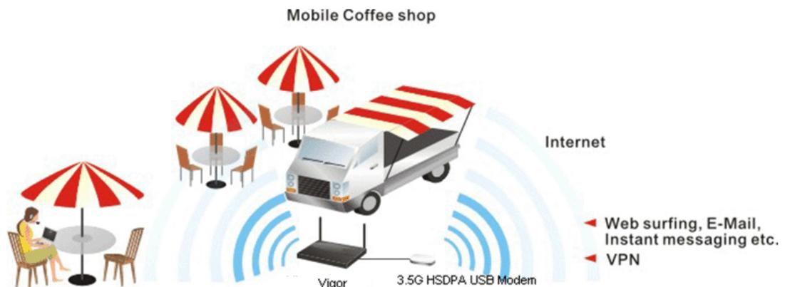
After connecting into the router, 3G USB Modem will be regarded as the second WAN port. However, the original Ethernet WAN1 still can be used and Load-Balance can be done in the router. Besides, 3G USB Modem in WAN2 also can be used as backup device. Therefore, when WAN1 is not available, the router will use 3.5G for supporting automatically. The
