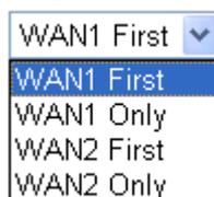
**WAN1 First** - While connecting, the router will use WAN1 as the first channel for VPN connection. If WAN1 fails, the router will use another WAN interface instead.
