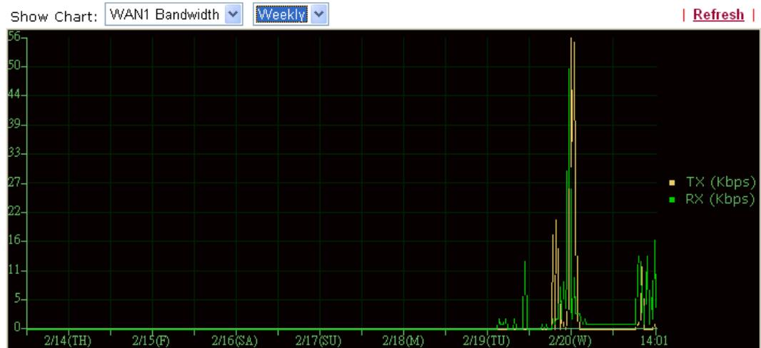
The horizontal axis represents time. Yet the vertical axis has different meanings. For WAN1/WAN2 Bandwidth chart, the numbers displayed on vertical axis represent the numbers of the transmitted and received packets in the past.
