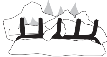
Figure 21 - Correct Burner Flame Pattern
