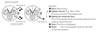
Please note: \* Following ②, further intervals or intermediates can be displayed by pressing push-button B. (Display interval, make up measured time, ...)
