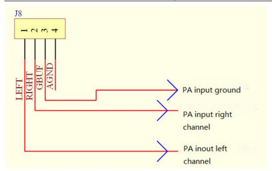
Notes: When amplifier board and MP3 module share the same low level power, you can not use the second way. For example, there is switching power supply of 12V and 5 V which share the same ground, you should use the first way to guarantee the potential of ground and etc.
